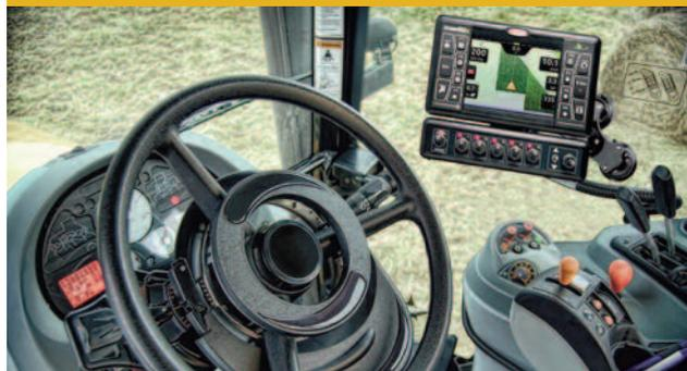
*manufacturers for all components and management systems; CAN is another acronym for Controller Area Network, an international standard designed to allow microcontrollers and devices to communicate with each other within a vehicle without a host computer. ISOBUS communications are thus based on the ISO 11783 international standard: "Tractors and machinery for agriculture and forestry – Serial control and communications data network".*
